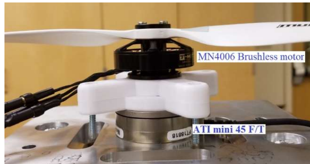
Figure 6.20. T-Motor MN4006 AntiGravity Brushless motor and Multistar Timber T-Style Propeller 13x4.4 mounted to an ATI mini-45 6-axis F/T sensor.
