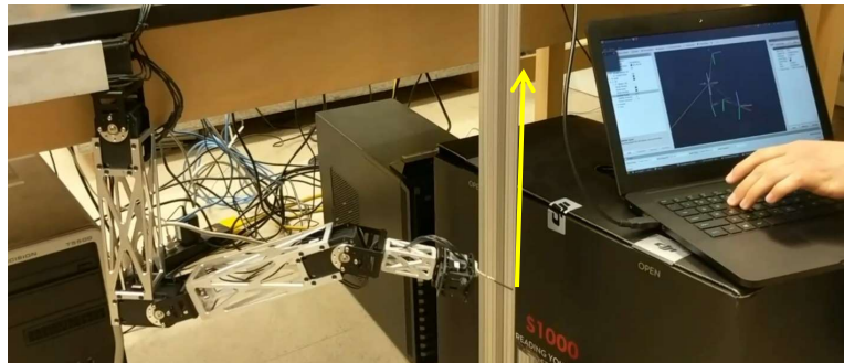
Figure 6.38. Cartesian control of a 3R manipulator. The manipulator is controlled via reference command of end-effector tip position.
