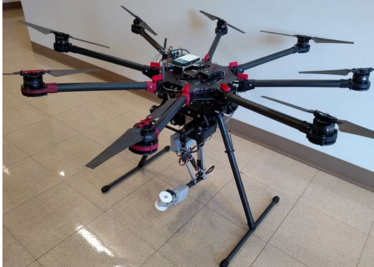
Figure 7.1. Octocopter aerial manipulator platform setup with plug-and-play sensor and manipulator peripherals.
